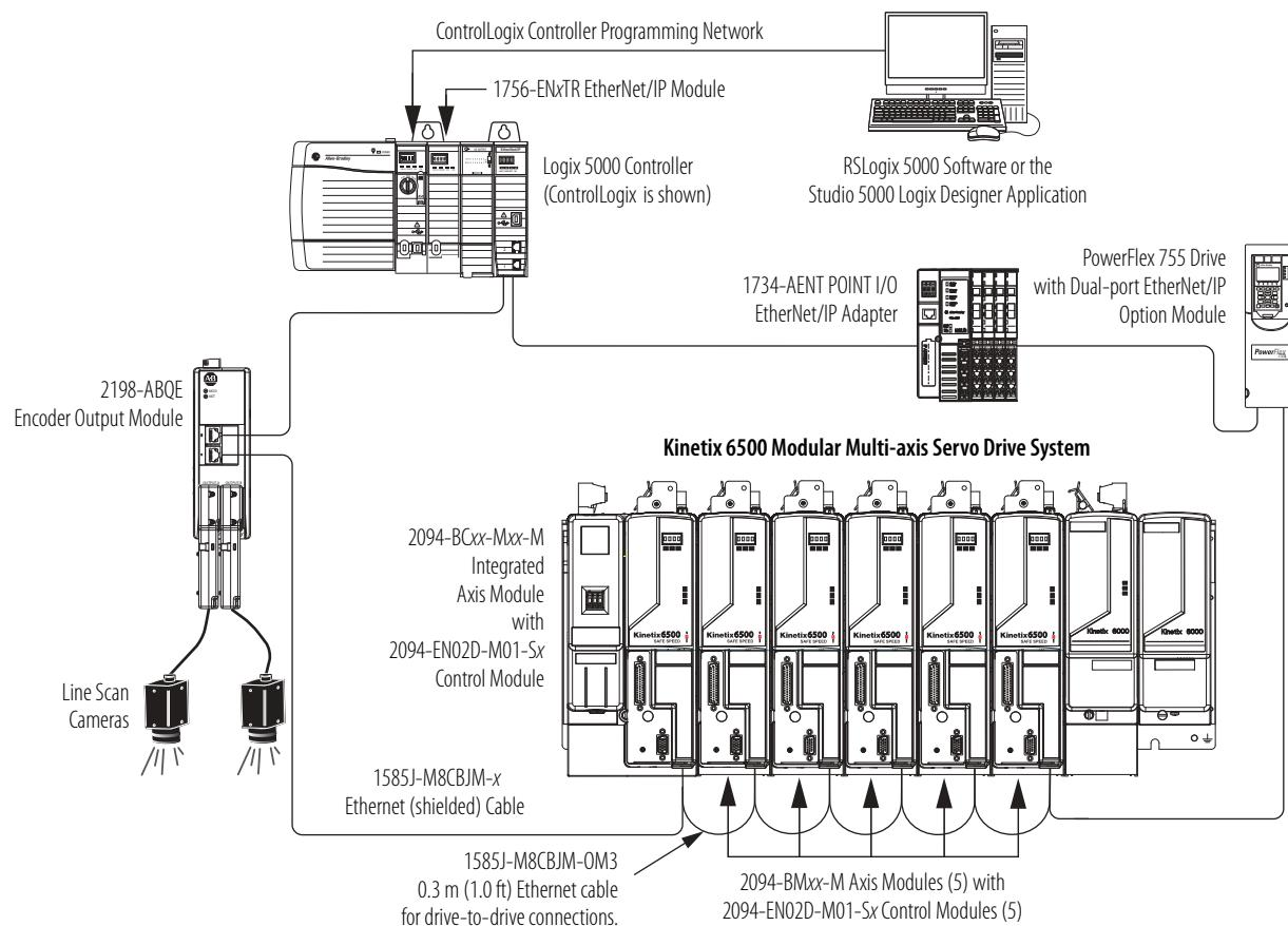
In this example, the devices are connected by using star topology. Each device is connected directly to the switch.
