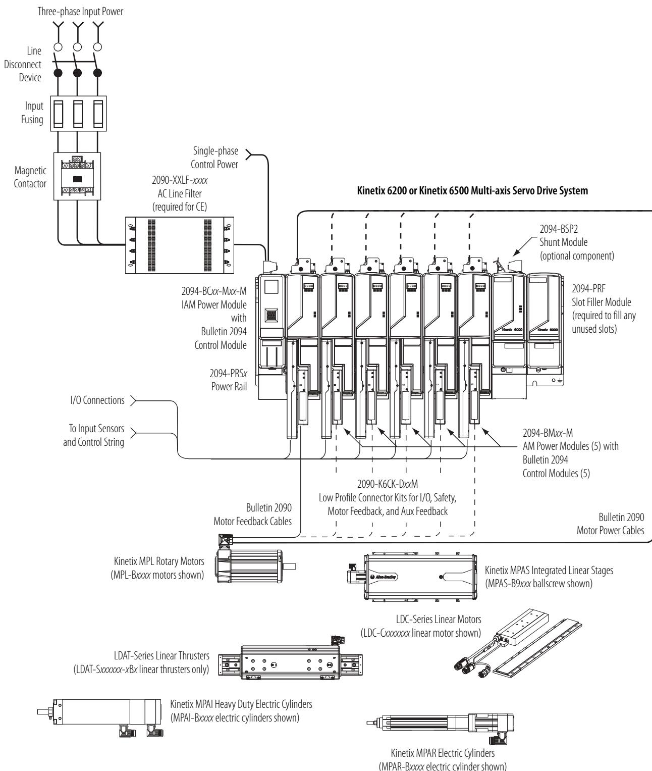
In this system configuration, the leader IAM power module is connected to the follower IAM module via the DC common bus. When planning your panel layout, you must calculate the total bus capacitance of your DC common bus system to make sure that the leader IAM power module is sized sufficiently to pre-charge the entire system. Refer to the Kinetix 6200 and Kinetix 6500 Modular Servo Drive User Manual, publication [2094-UM002](#), when making this calculation.
