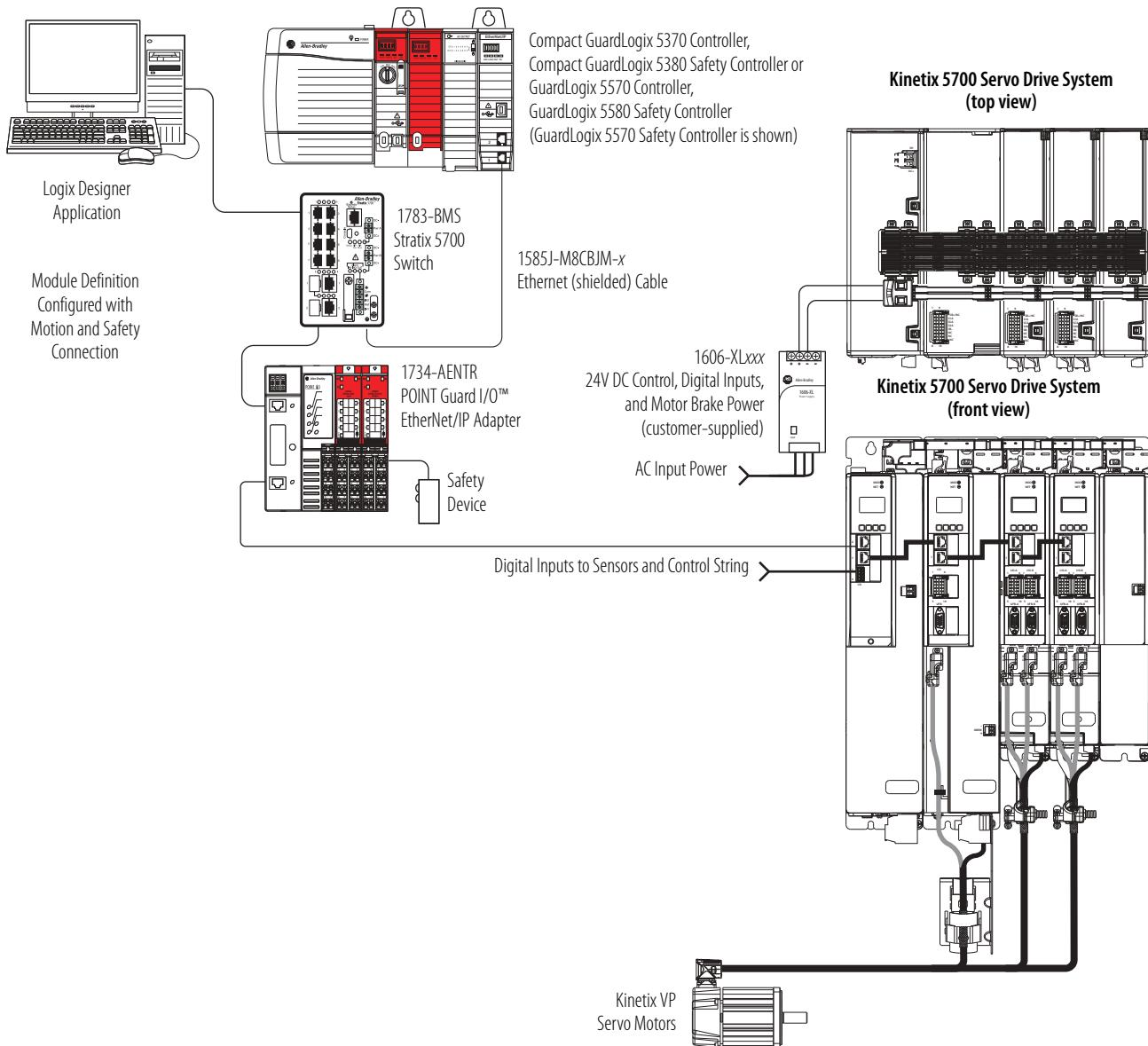
In this example, a non-safety controller makes the Motion Only connection and a separate GuardLogix safety controller makes the Safety Only connection.
