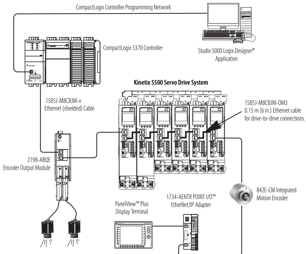
In this example, the devices are connected by using ring topology. If one device in the ring is disconnected, the rest of the devices continue to communicate. For ring topology to work correctly, a device level ring (DLR) supervisor is required (for example, the Bulletin 1783 ETAP device). DLR is an ODVA standard.
