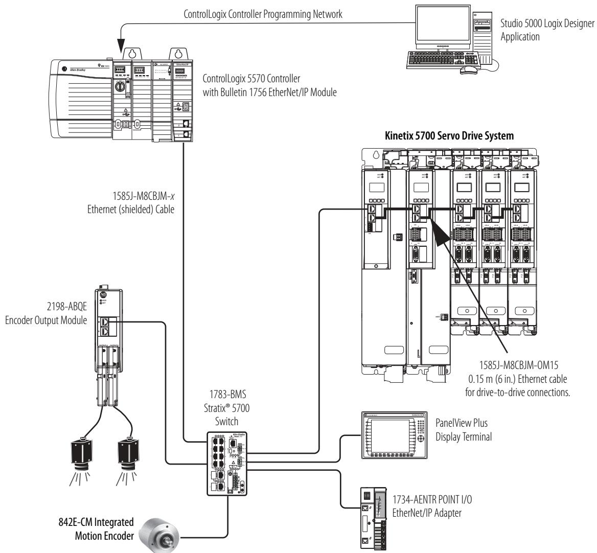
You can use the 842E-CM integrated motion encoder for applications requiring an external encoder for gearing or camming to the Kinetix 5700 drive. By providing auxiliary feedback directly through the EtherNet/IP network, the 842E-CM encoder helps eliminate the need for point-to-point wiring while letting customers use the encoder in a variety of network topologies. For more information, see the 842E-CM Integrated Motion on EtherNet/IP Product Profile, publication [842ECM-PP01](#).
