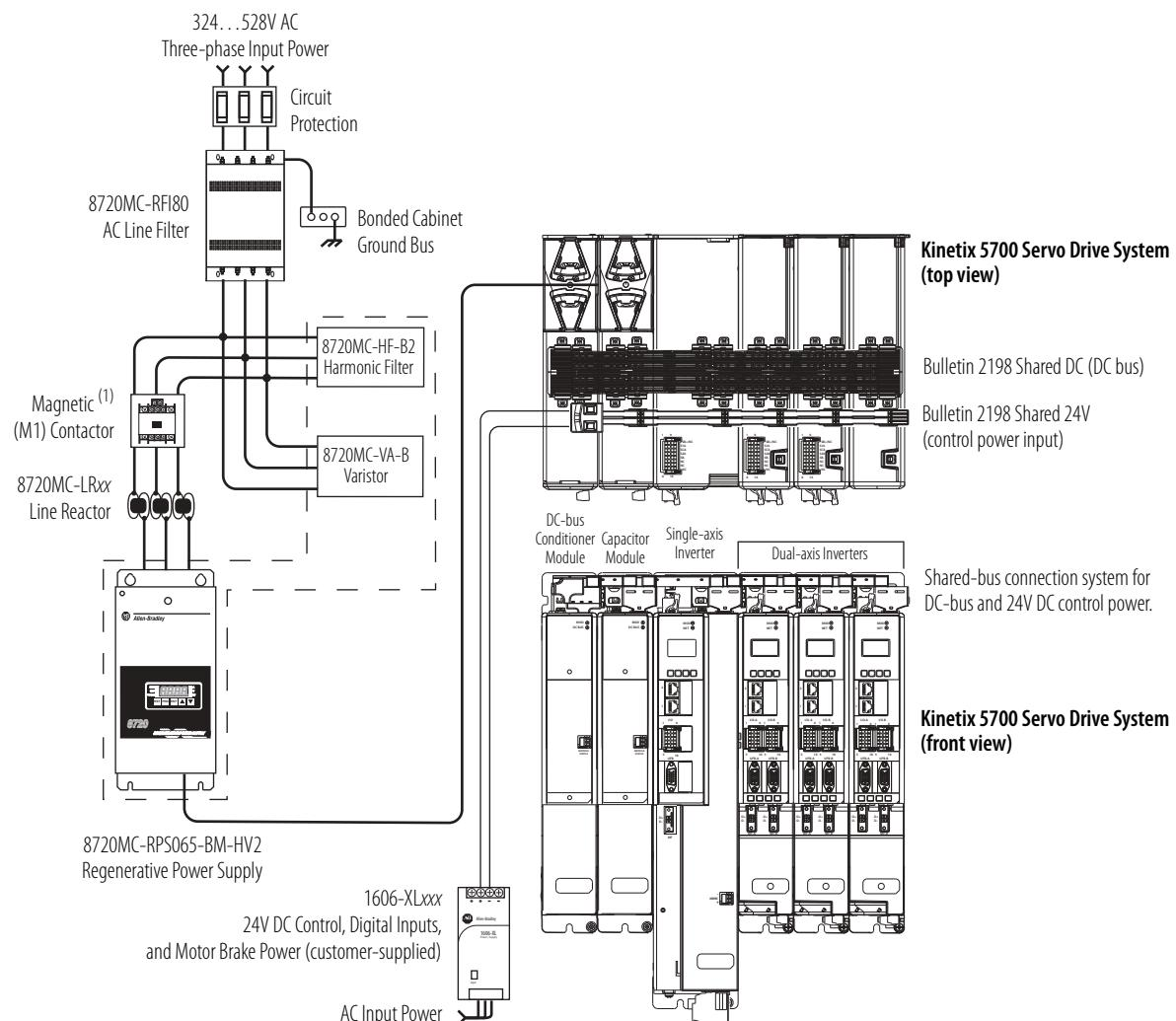
(1) This M1 contactor is controlled by the 8720MC regenerative power supply.
