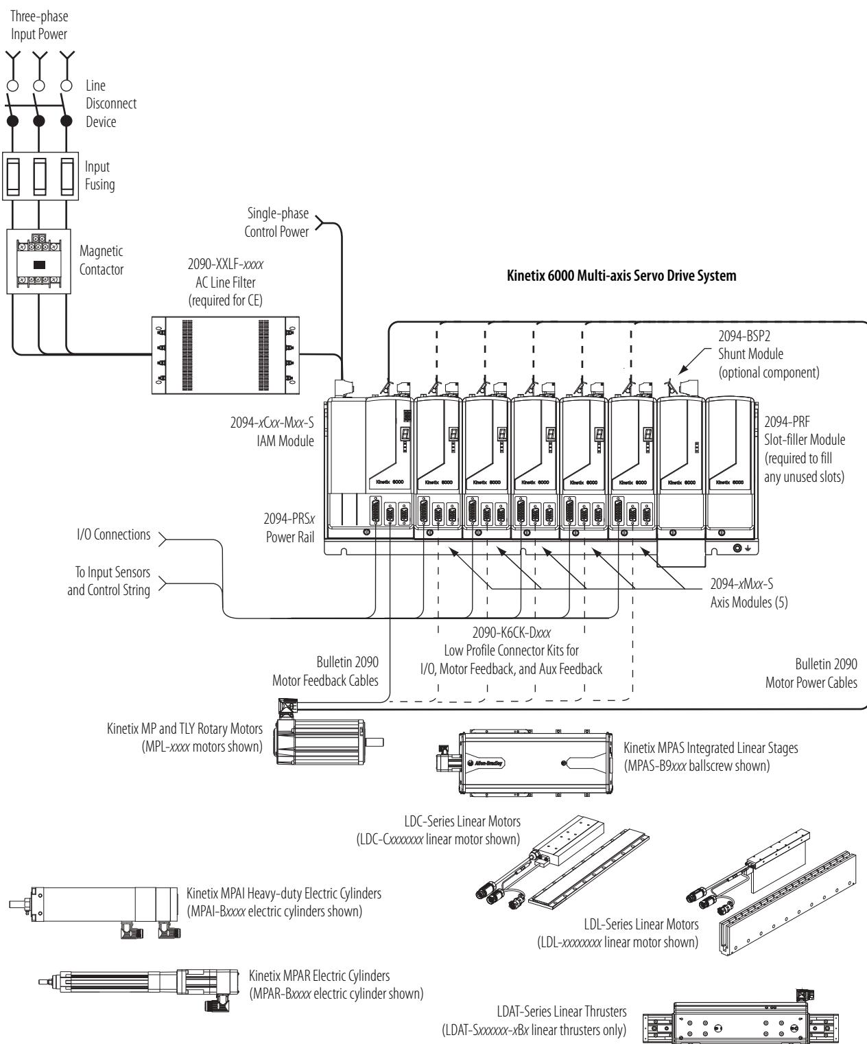
In this system configuration, the leader IAM module is connected to the follower IAM module via the DC common bus. When planning your panel layout, you must calculate the total bus capacitance of your DC common bus system to make sure that the leader IAM module is sized sufficiently to pre-charge the entire system. Refer to the Kinetix 6000 Servo Drive User Manual, publication [2094-UM001](#), when making this calculation.
