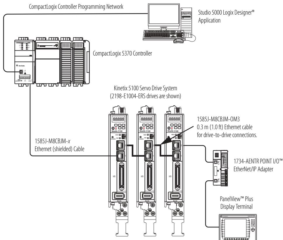
In this example, the devices are connected by using ring topology. If only one device in the ring is disconnected, the rest of the devices continue to communicate. For ring topology to work correctly, a Device Level Ring (DLR) supervisor is required (for example, the Bulletin 1783 ETAP device). DLR is an ODVA standard. For more information, refer to the EtherNet/IP Embedded Switch Technology Application Guide, publication [ENET-AP005](#).
