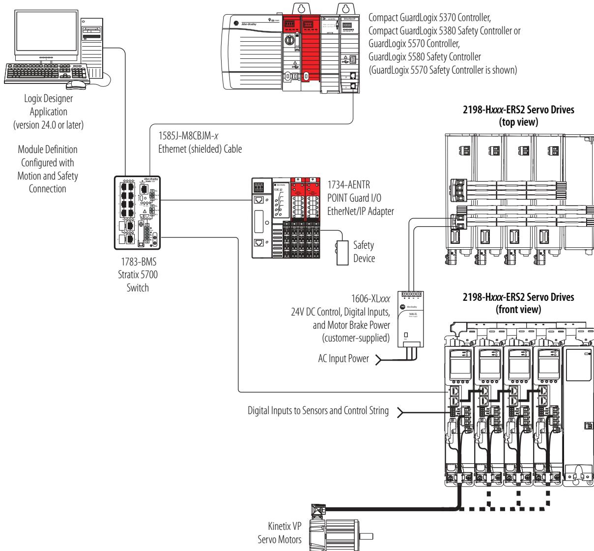
In this example, a non-safety controller makes the Motion-only connection and a separate GuardLogix safety controller makes the Safety-only connection with the 2198-Hxxx-ERS2 drives.
