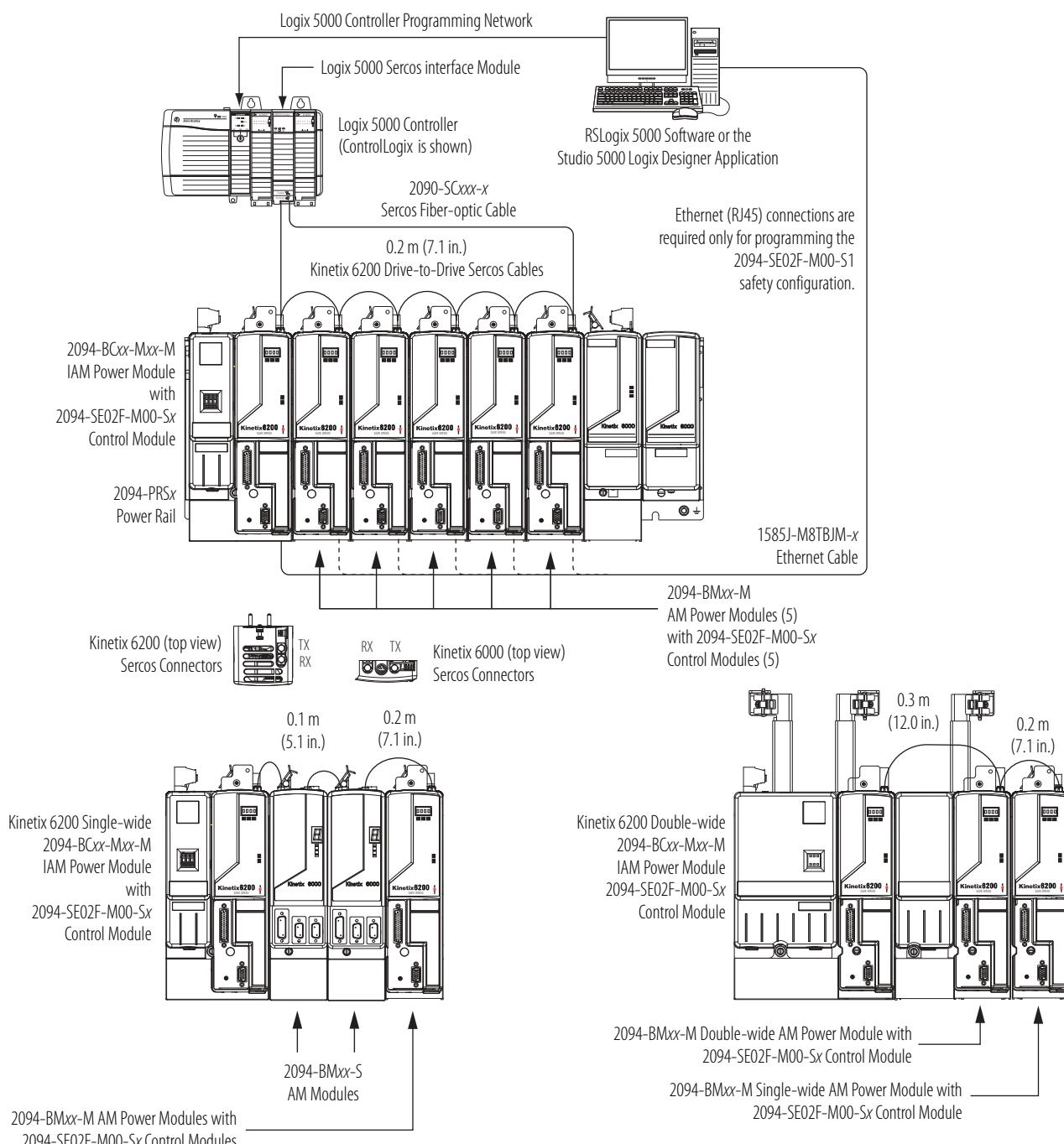
The Kinetix 6500 control modules support any Ethernet topology including linear, ring, and star by using ControlLogix, GuardLogix®, or CompactLogix controllers. These examples feature the ControlLogix 5570 programmable automation controllers with support for integrated motion and integrated safety over the EtherNet/IP network. Other Allen-Bradley® controllers are also compatible with the Kinetix 6500 servo drives.
