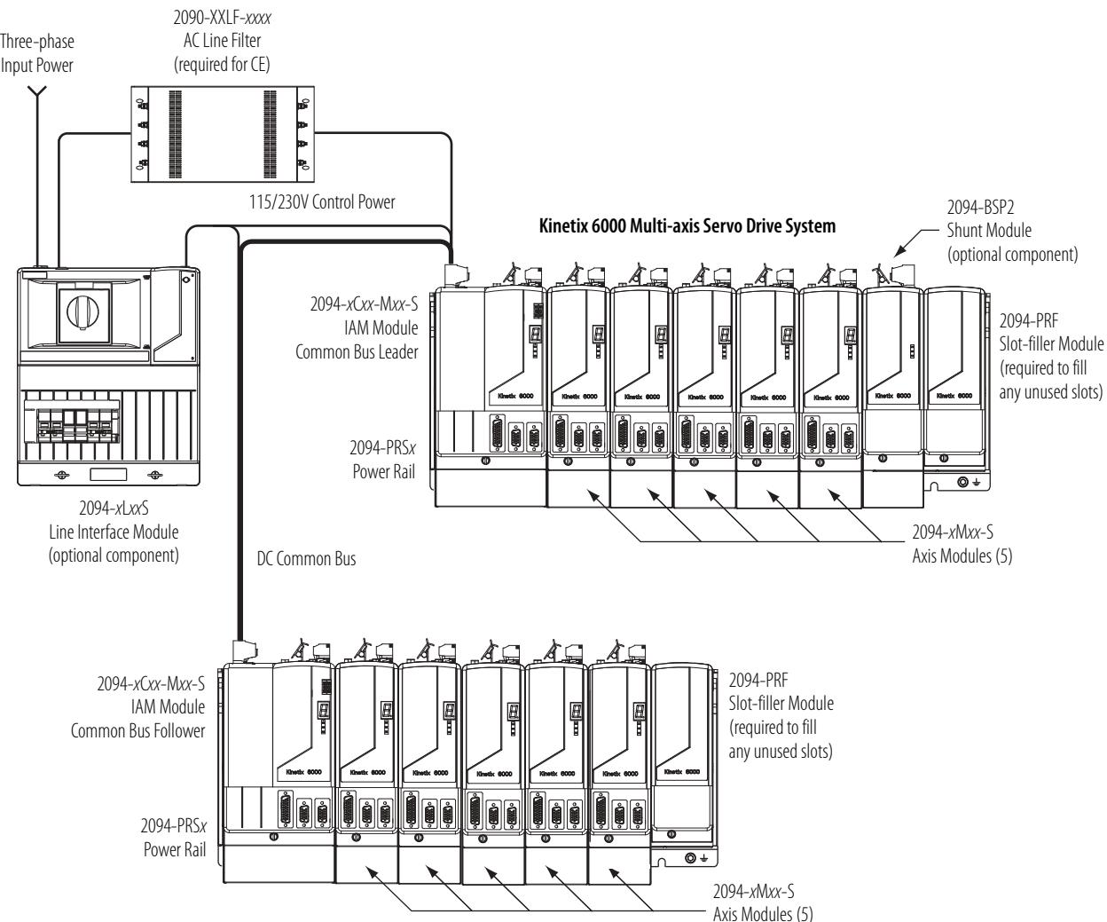
Motors and other details common to both three-phase AC and DC common-bus configurations are removed.
