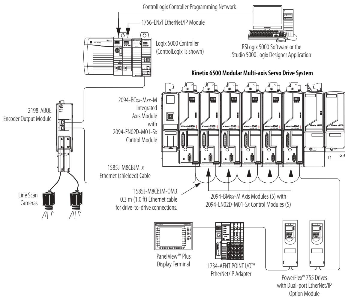
In this example, the devices are connected by using ring topology. If one device in the ring is disconnected, the rest of the devices continue to communicate. For ring topology to work correctly, a device level ring (DLR) supervisor is required (for example, the Bulletin 1783 ETAP device). DLR is an ODVA standard.
