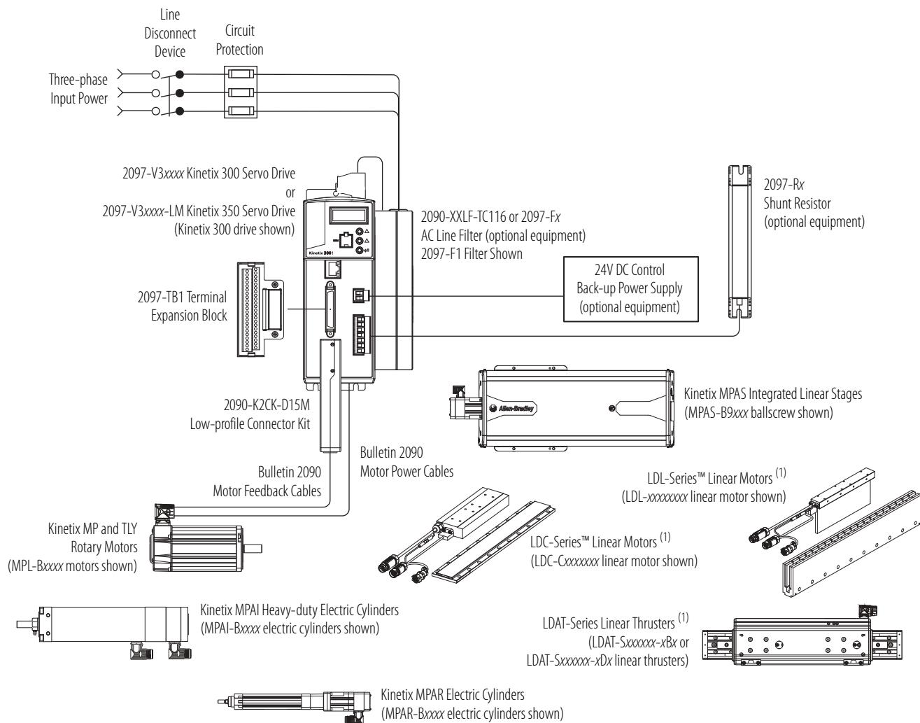
(1) LDC-Series and LDL-Series linear motors, and LDAT-Series linear thrusters are compatible with only Kinetix 300 servo drives.
