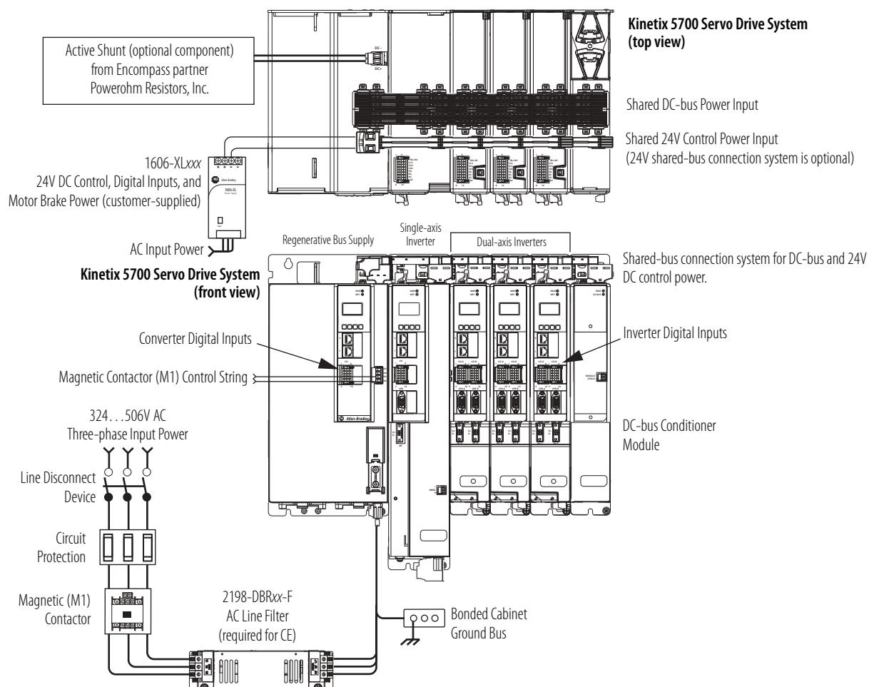
In this example, the 2198-RP312 regenerative bus supply is mounted on the far right and followed by the 2198-S312-ERSx single-axis inverter, and two 2198-D020-ERSx dual-axis inverters.
